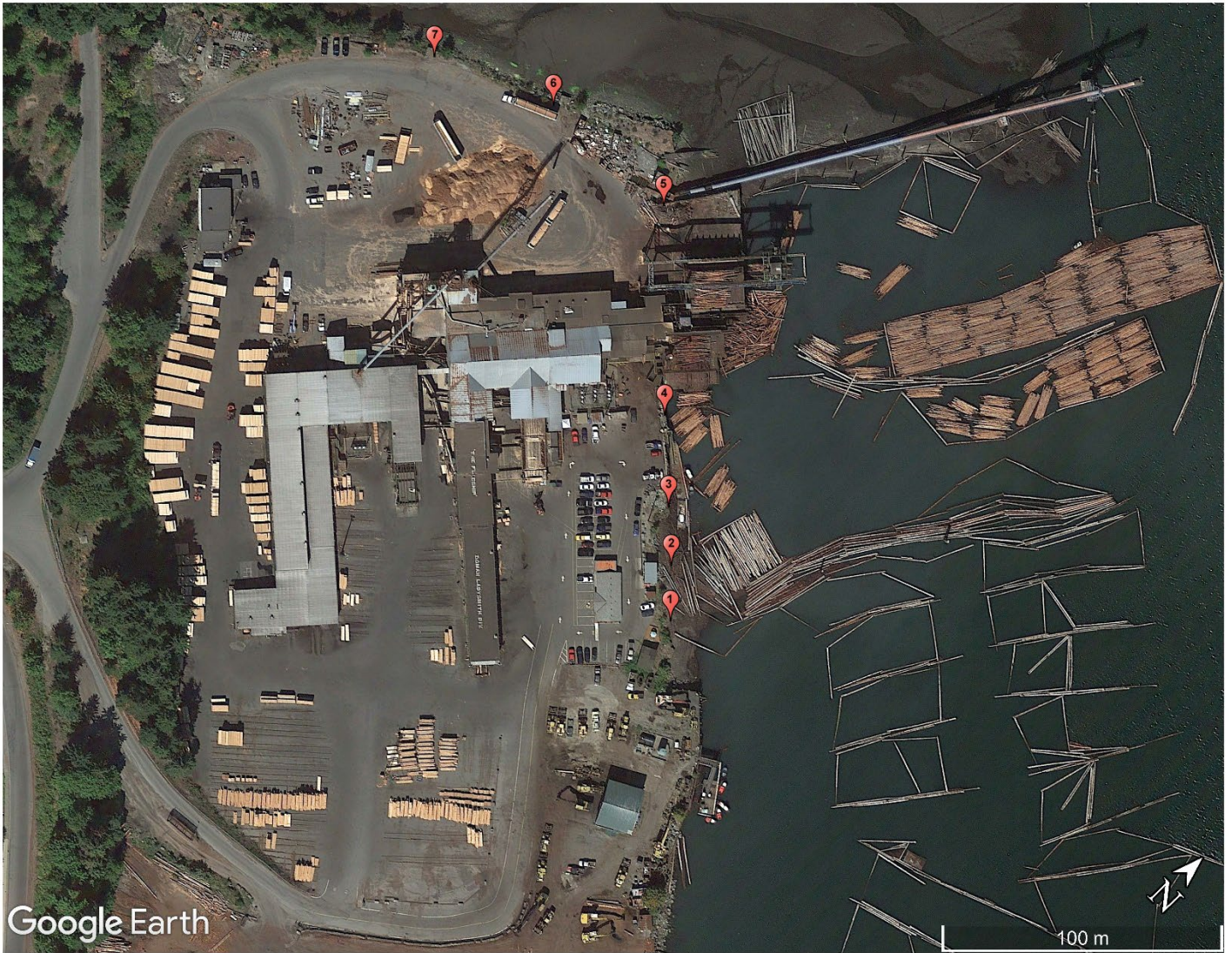
Figure 1. Overview of the Ladysmith sawmill. Effluent discharge locations are identified by the red balloons.
