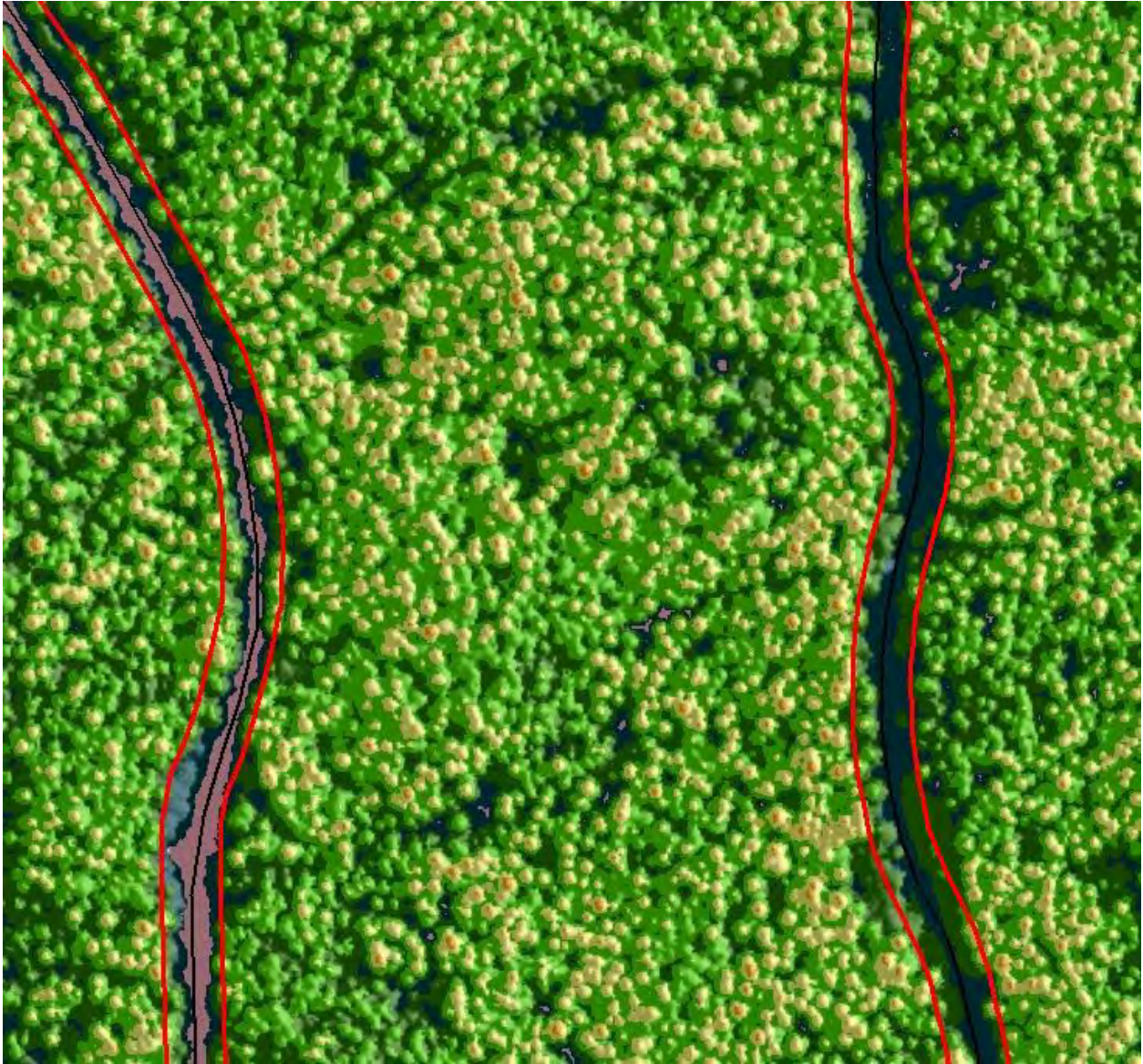
Figure 26 – Road buffer with crown height model
